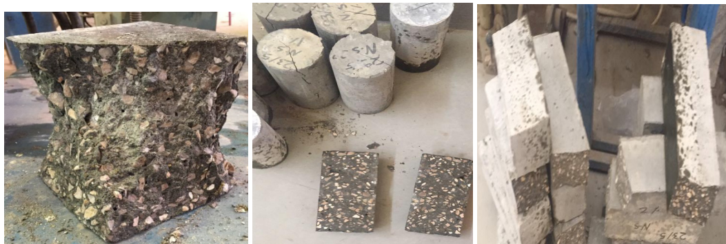
Fig. 7. Concrete cubes, cylinders and prisms after testing
